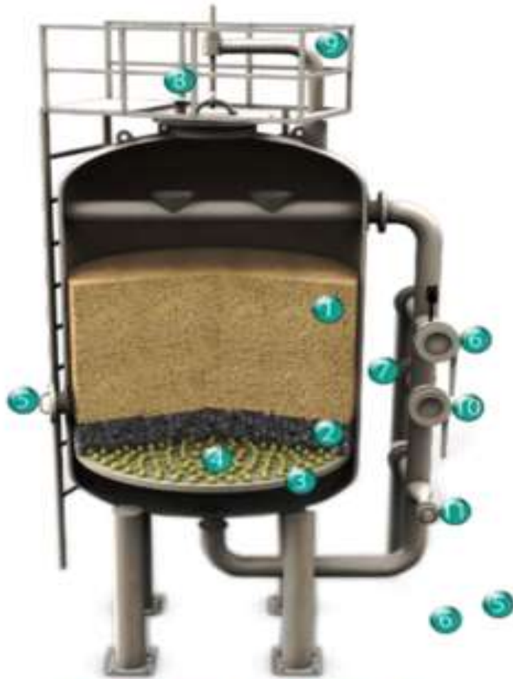
Pressure Sand Filter
